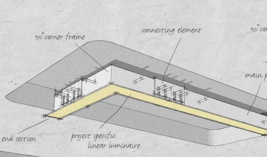
The shape and length of the light lines are specified during the planning of this lighting solution in the structural engineering phase. The light and luminaire design can be individually adapted and, thanks to the magnetic holders, can also be subsequently altered if desired.
