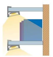
All aluminium profiles and covers are subject to certain length tolerances. This is +20/-0 mm irrespective of the length, i.e. a profile has at least the specified length, but can be up to 20 mm longer.
