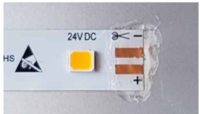
Fig. 2: Liquid rubber on the cut edge
